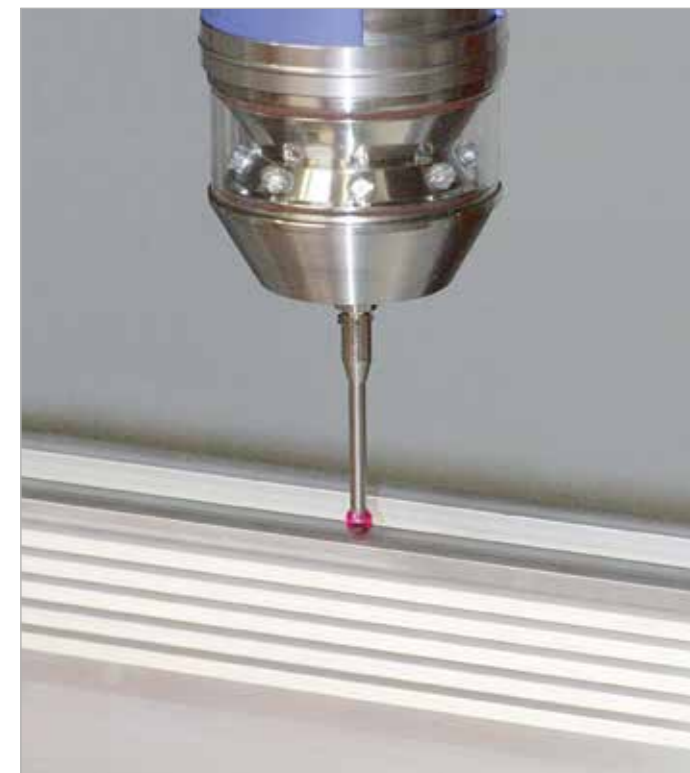
Measuring with a 3D probe. This allows exact positioning of machining operations even with existing profile tolerances.
