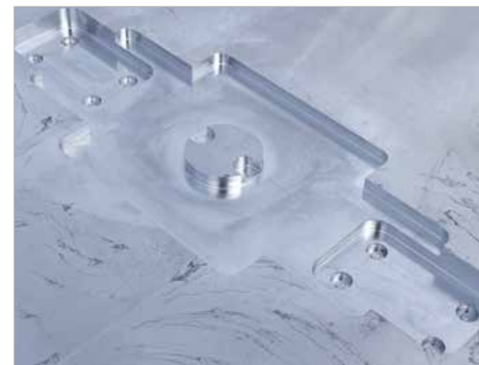
The “Free-form removal” function automatically computes the milling paths required to complete full-surface removal for the specified free form. During the removal process, previously defined “islands” can be left alone.
