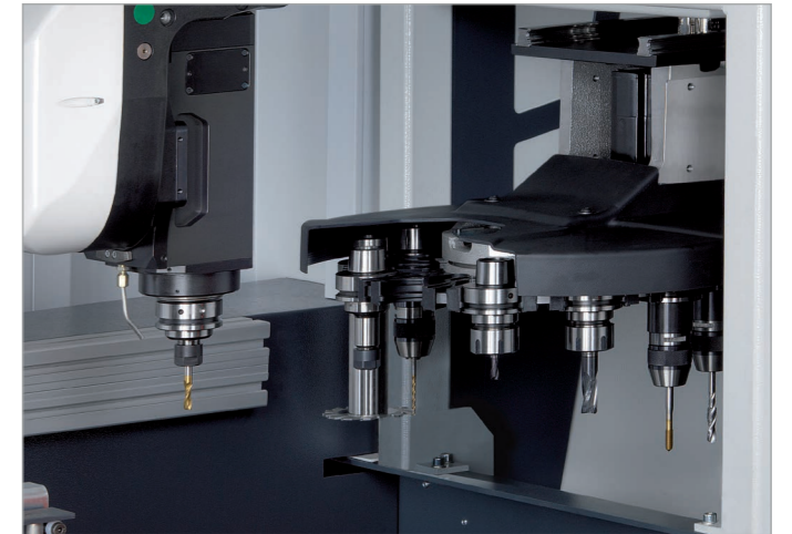
Rotating magazine with 12-fold tool changer
