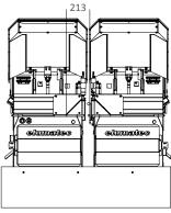
Minimum dimension for 45° cut with short stroke stop on the travelling unit: 213 mm
