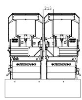
Minimum dimension for 45° cut with short stroke stop on the stationary unit: 213 mm
