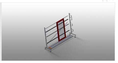
Vertical roller conveyor for transportation and storage of window elements
