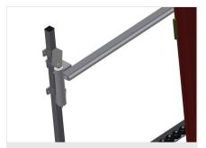
Support Rear support with plastic slide bars, top and bottom
