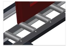
**Support rollers**Rollers throughout, support roller width, 200 mm.
