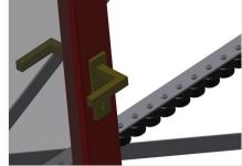
**Mini-roller conveyor**Three mini-roller conveyors with rubber rollers, diameter 50 mm
