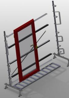
Vertical roller conveyor for transportation and storage of window elements
