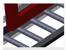
Support rollers Rollers throughout, Roller conveyor divided into three parts, 3x 120 mm. Roller conveyor units, 2,000 mm, 3,000 mm and 4,000 mm long
