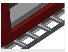
Profile protectors Profile protectors for support rollers 200 mm (Alum./11 x, Alum./16 x and Alum./21 x). Support rollers covered with protective tubing
