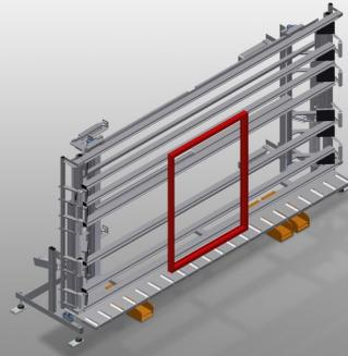
Inspection and glazing unit for glazing and final inspection in individual and serial assembly line production
