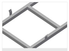
Safety tabs Safety tabs to secure the pallets
