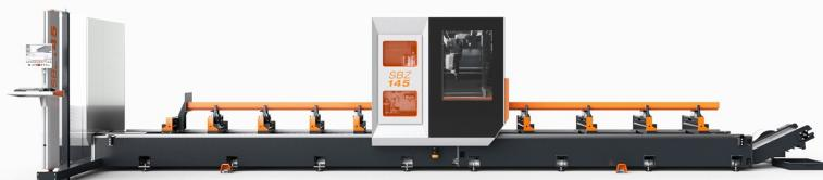
Designed for the requirements of metal construction and industrial use, the SBZ 145 with its 5 processing axes offers a processing area of 560 mm x 350 mm x 7,500mm. Equipped with an autonomous clamping axis and a generously designed tool magazine for milling cutters, drills, thread cutters and saw blades. The SBZ 145 has numerous processing options for cutting from the profile bar with processing or optionally in pendulum operation with processing of pre-cut individual parts (2x 3.250mm).
