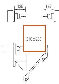
**Machining area, Y and Z-axes**
