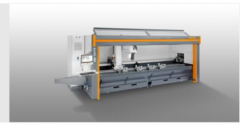
Designed for economical and efficient machining of aluminium, PVC and thin-walled steel profiles
