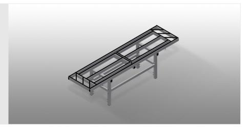
Assembly station for all assembly tasks on special-order elements and curtain walls
