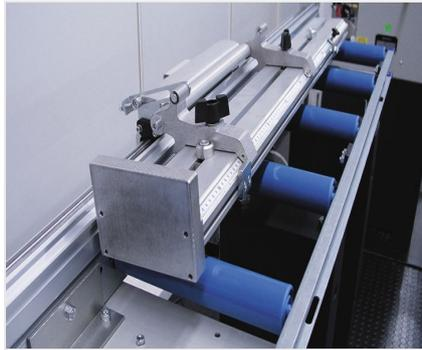
**Stop and measurement system MMS 200**
