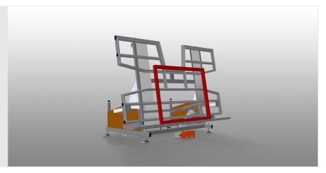
Assembly table for vertical and horizontal assembly
