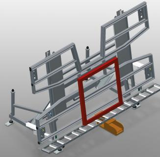
Assembly table for vertical and horizontal assembly
