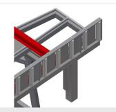
Roller support Roller conveyor can be lowered pneumatically to allow unhindered working in horizontal position; in vertical position, trouble-free onward transport is possible
