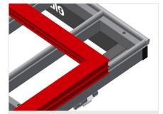
**Supporting surfaces**Supporting surfaces with plastic slide bars
