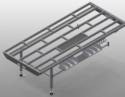
Modular work table for a production line (basic module)
