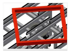
Lift and turn mechanism Practical for hardware assembly as well as for final assembly and gasket insertion. Inner table height pneumatically adjustable. Inner table can be rotated; with pneumatic fixing brake
