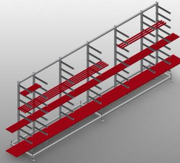
Stable steel construction. Glazing bead rack for horizontal storage of aluminium and plastic glazing beads. Ideal for storing and sorting glazing beads, e.g. before the glazing bead saw. Seven support arms are evenly spaced along the rack. Four centre supports are adjustable. Nine support arms are freely adjustable, giving variable support arm spacing. Support arms are rubber coated. Well-organised storage provides quick access.
