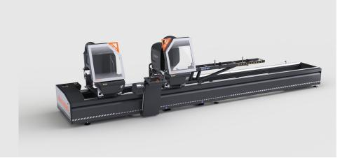
Double mitre saw with automatic length adjustment of the moving head by brushless motor. Pneumatic tilting of the sawing unit from  $90^{\circ}$  to  $45^{\circ}$  or  $22^{\circ}30'$  by two fixed positions. Optionally with mechanical adjustment of the intermediate angle. Hydropneumatic saw blade feed.
