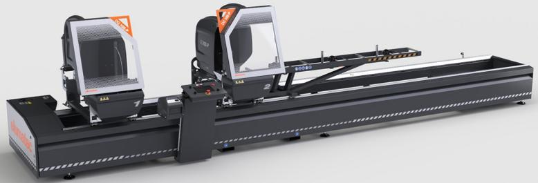
Electronic twin-head cutting-off machine with automatic traverse of the moving cutting head powered by brushless motor with numerical control system. Pneumatic control of the angular setting from 90° to 22°30' (external) in two fixed positions or with optional mechanic adjustment of intermediate angles. Hydro-pneumatic blade feed.
