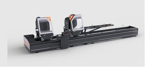
Electronic twin-head cutting-off machine with automatic traverse of the moving cutting head powered by brushless motor with numerical control system. Pneumatic control of the angular setting from 90° to 22°30′ (external) in two fixed positions or with optional mechanic adjustment of intermediate angles. Hydro-pneumatic blade feed.
