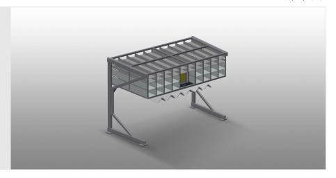
Hardware rack with 36 compartments for orderly hardware storage at the sash assembly station
