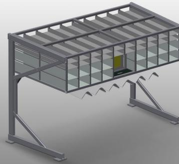
Hardware rack with 36 compartments for orderly hardware storage at the sash assembly station
