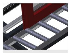
Support rollers Rollers throughout, support roller width 3x 120 mm.Roller conveyor unit, 4,000 mm long
