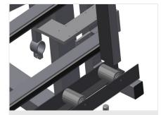
**Pressing bar**Pneumatic centring. Precision ensured through parallel clamping bar pressing technique
