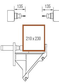
**Machining area, Y and Z-axes**
