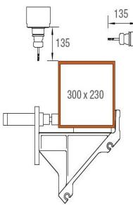
**Machining area, Y and Z-axes**
