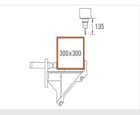
Machining area, Y and Zaxes Profile machining from above
