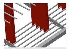
Supporting surface Supporting surface with bar grid floor
