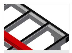
Rubber strips Supporting surfaces with rubber-knob profile
