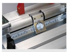
Stop and measuring system MMS 200
