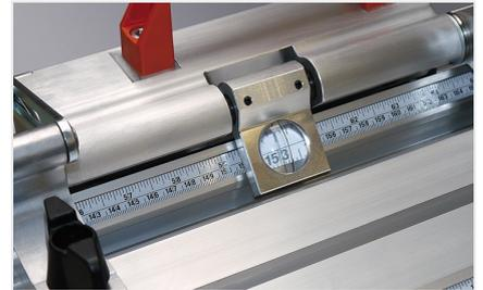
**Stop and measuring system MMS 200**
