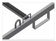
Forklift openings and crane attachment points
