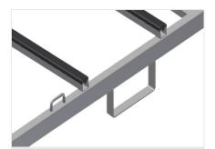
Forklift openings and lashing strap attachment points
