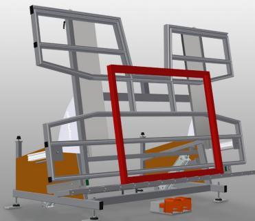
Assembly table for vertical and horizontal assembly
