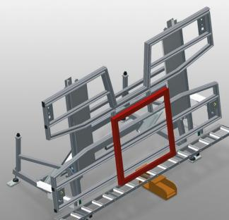
Assembly table for vertical and horizontal assembly
