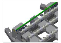
**Supports**Lower supporting surfaces with lifting rollers for easier loading and unloading
