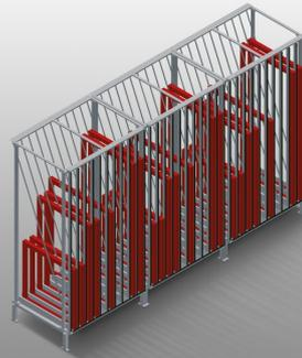
Rack for storage of window elements. Stable steel construction. Vertical sash sorting rack for sorting the sash elements. Sorting rack with ten compartments. Fast access to the elements. Plastic-coated compartment dividers. Supporting surface with plastic sheet. Special slide plate bearing surfaces enable ergonomic removal of the sash elements as needed.
