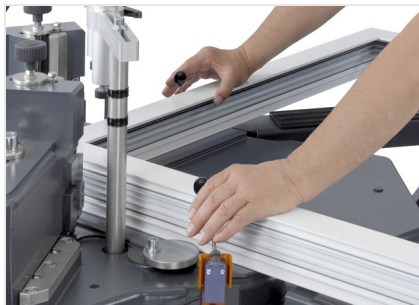
Corner crimper EP 124/20 2-hand operation
