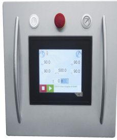
E 390 Positioning control
