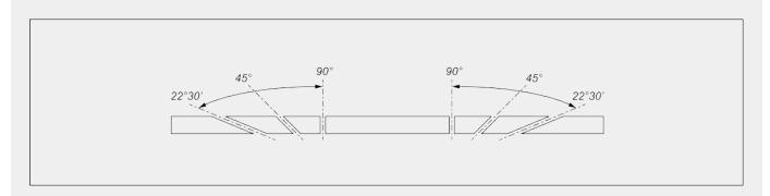
Mechanical adjustment of intermediate angles
